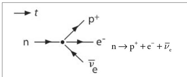
Fig. 2. Diagram of  $\beta^-$  decay.
